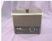
One common method is to place the wafer in acetone and use an [ultrasonic cleaner](#) for some period of time (typically 5 to 15 minutes). Immediately after removal, rinse with ethanol and/or methanol and dried with a dry N2 gun, or a compressed [air can](#). When using this method, you must watch for residue left on the surface by the solvents
