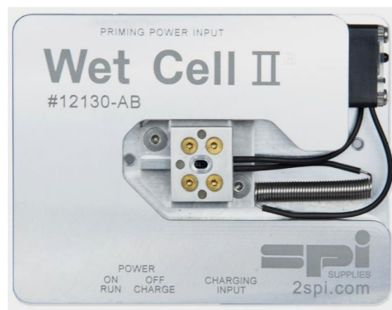
Figure 1. Top view of Wet Cell II
