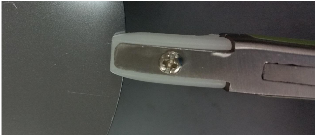
Fig. 1H – It is important when cleaving to grip the substrate as close to the edge as possible to ensure a clean break along the crystal orientation.
