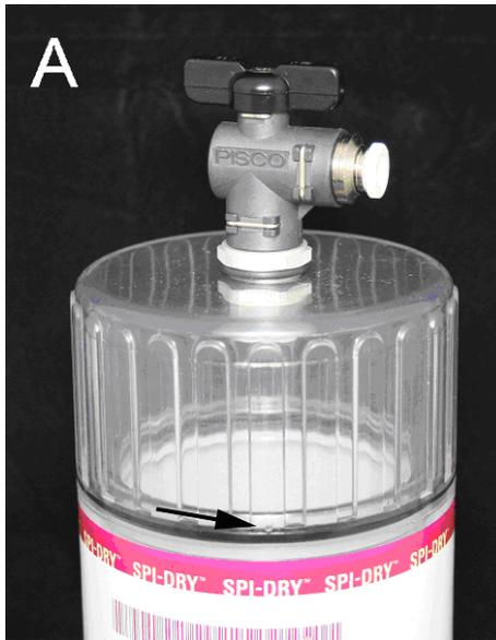
5. Stop the flow by further turning the lower portion of the Sample Preserver capsule until the body o-ring is just above the hole in the upper portion as shown by the arrow in Figure 1B.
