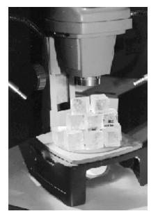
The cleaving produces a very flat, relatively clean surface. However, it must be prepared immediately and then placed in the vacuum chamber of the system being used for the deposition, followed by an immediate pump down, which is then followed by the deposition of one or more thin film coatings. If all of this is not done quickly and as described some of the benefit of the freshly cleaved surface could be lost.
