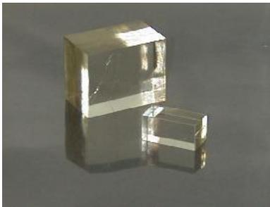
The procedure is to place the blade parallel to one of the existing edges, and then tap lightly with the small hammer. Cleaving occurs instantly and the only time there is a problem is when the razor blade being used gets dull (it should be changed after every several cleavings). In practical terms, a 2 mm thick slab is probably the lower limit in thickness that can be obtained this way.
