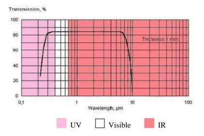
MgO single crystal transmission spectrum demonstrating the high transmittance over both the UV and the IR ranges. The light purple color to the left is UV and the light red color to the right is considered IR. The "white" region is the visible point of the spectrum.
