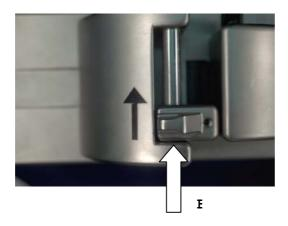
4 Break the knife by pushing the breaking lever (C) slowly upwards. Remove the knife for examination on the knife tray .
