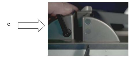
5 Before making more knives all traces of glass flakes and debris should be removed from the knife maker surfaces using the brush.
