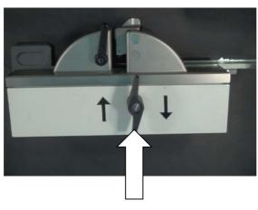
3 Score the glass by pulling or pushing the scoring assembly (B) over the glass towards the clamping leaver using your index finger or thumb with a consistent speed. Never score the glass in both directions.
