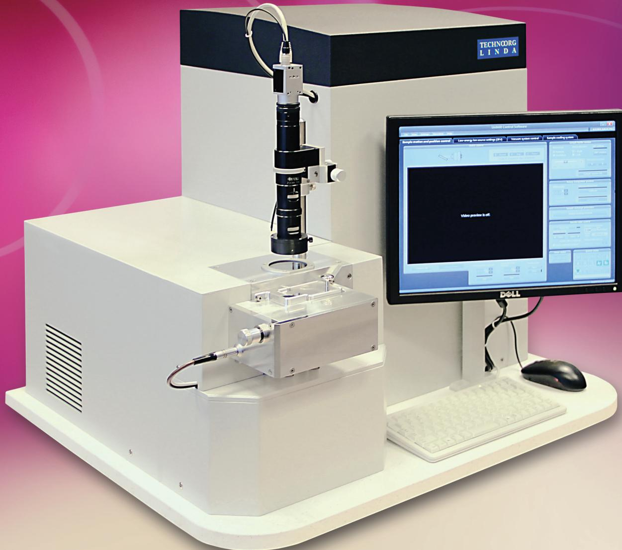
The IV7 Universal Ion Mill is recommended to users developing new materials or new sample preparation methods. Due to its extremely high milling rate, it is optimal for studying hard-to-sputter materials, such as diamond, sapphire, etc. Its exclusive
