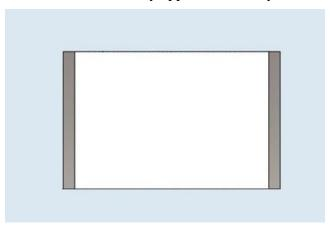
There are a number of different qualities of the busbar that one could apply. As a standard product, we offer the slides with a silver line silk screened on at the edge (or elsewhere is desired) that exhibits, when cured and dried, exhibits a surface resistivity of better than 0.2 ohms / square. The busbar is typically three micrometers in thickness with a three millimeter width.
