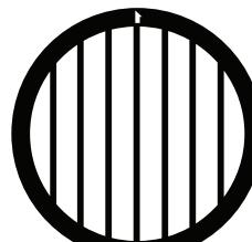
**Parallel** grids allow you to take sequential micrographs without interference from grid bars.
