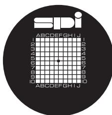
**Calibrated** grids are needed primarily by those doing work that must conform to the AHERA specifications.
