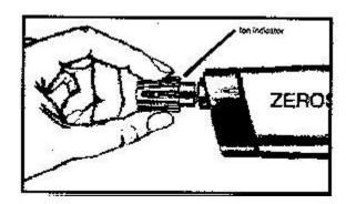
Hold the Zerostat within 12" (30.5 cm) of the surface or object to be treated. Squeeze the trigger slowly for about two seconds, to emit a stream of positive ionized air over the surface of the object. As the trigger is slowly released, a negative show of air ions is produced resulting in static neutralization. Repeat this procedure at several points across the surface of the object.
