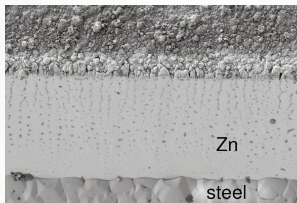
Cross-sectional specimen of Zn coated steel was prepared by ion beam slope cutting process cut into the near surface layer of the bulk sample
