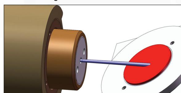
To produce samples for Electron Back Scatter Diffraction (EBSD) study and Orientation Imaging Microscopy (OIM)
