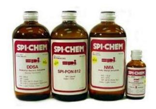
hardness, to match the embedded material, can be made by varying the proportions of DDSA (softener) and NMA (hardener). It is well known that hard specimens in a soft resin block will tear away from the block, whereas soft specimen materials will section unevenly if embedded in a hard resin formulation. In addition to the wide range of hardness that is attainable, other advantages include improved penetration (in biological tissue), contrast, and ease of obtaining stable thin sections.
